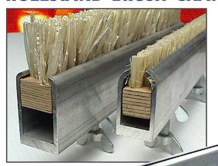
Brush blocks must be sized to fit snugly into the inside width of the aluminum brush channel. The large block is generally used for corrugated rolls; the small block for smooth rolls.
